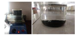
Hummer's method is a chemical process that can be used to generate graphite oxide through the addition of potassium permanganate to a solution of graphite, sodium nitrate and sulfuric acid. It is commonly used by engineering and lab technicians as a reliable method of producing quantities of graphite oxide. It is also able to be revised in the creation of a one-molecule-thick version of the substance known as graphene oxide.
