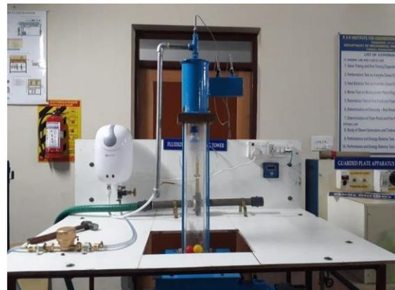
**Fig 1: Experimental setup of FBCT**
